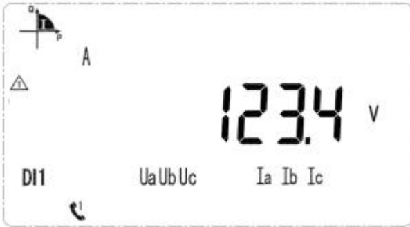
Voltage on A phase is 123.4V
