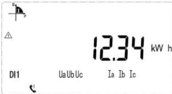
Current forward active energy 12.34kWh
