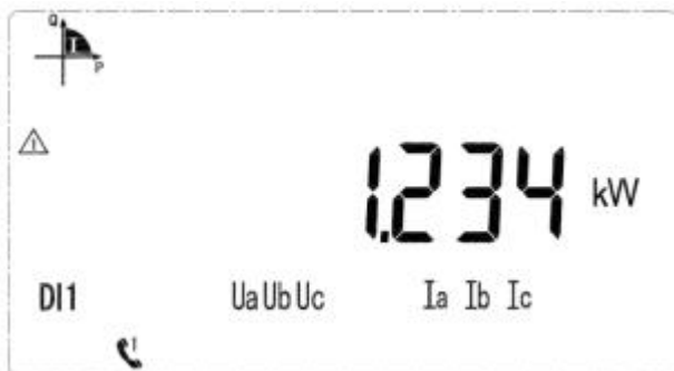
Current total power is 1.234kW
