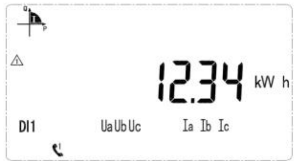
Current reversing active energy 12.34kWh
